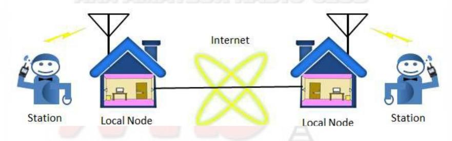
An amateur Radio operator calls a local Node's radio which is connected to the Internet via a PC. The local Node radio relays the amateur's call to the Internet via the PC. The PC relays the amateur call to another Node's PC that is also connected to the Internet, then send it to the Node radio. Then local Node radio then relays the call to the receiving amateur radio station.
