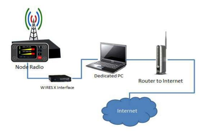
Figure shows a typical Local Node and its components. This is what it is needed to create the Local Node.
